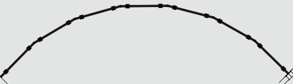
Curved and partially curved track configurations (min. radius 3 metres)
